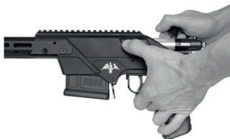
Pic. 2 Removal of the Bolt
